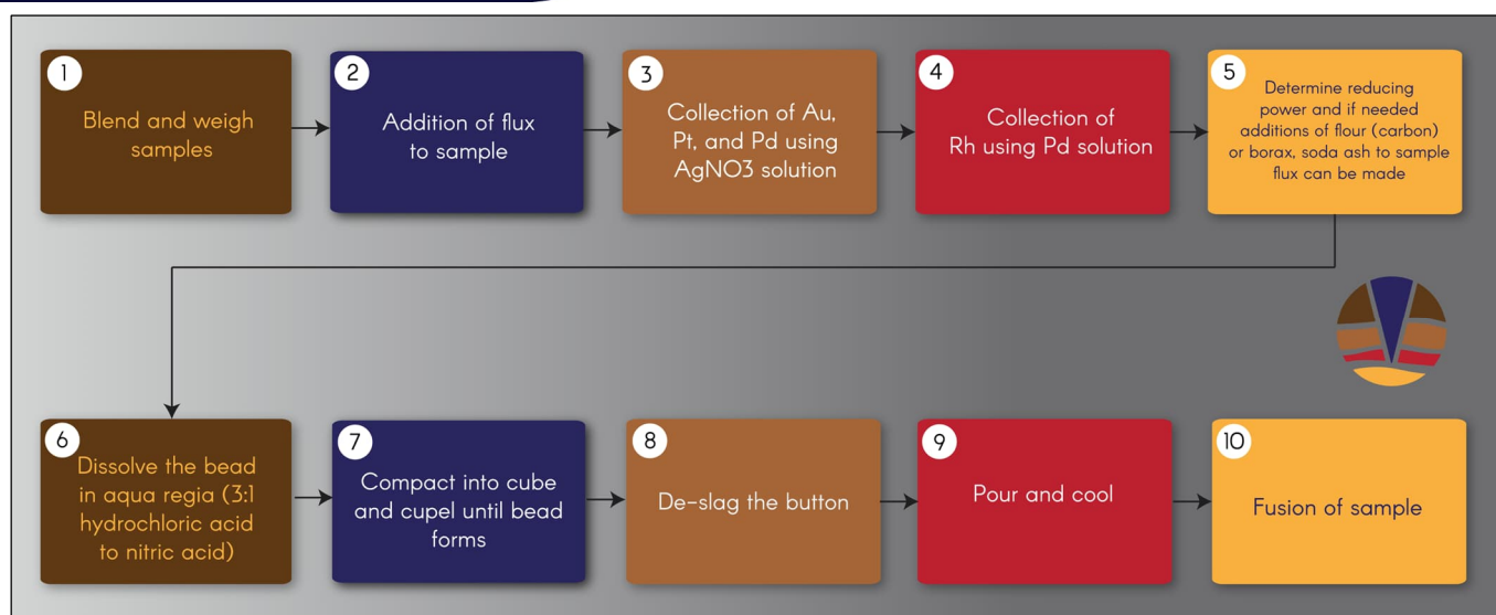
Figure 27. Flow chart for SGS sample preparations before conducting elemental determination methods.
