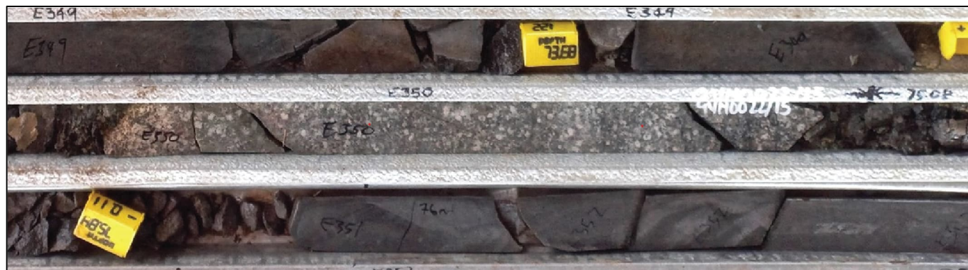
Figure 16. Photograph showing alkali-granite dyke intrusion into the Volspruit Reef.
